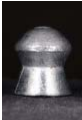
Calibre 0.22", Weight 14.6gn, Length 6.33mm, Skirt Dia. 5.68mm, Head Dia. 5.45mm
