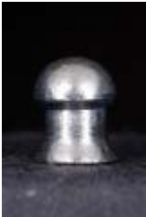
Calibre 0.177", Weight 7.50gn, Length 5.52mm, Skirt Dia. 4.55mm, Head Dia. 4.47mm
