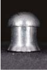
Calibre 0.22", Weight 14.0gn, Length 6.50mm, Skirt Dia. 5.70mm, Head Dia. 5.48mm, BC 0.027
