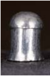
Calibre 0.22", Weight 18.0gn, Length 7.50mm, Skirt Dia. 5.80mm, Head Dia. 5.52mm
